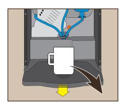
Remove the rinsing cup and drip pan, and rinse under running water. Reinstall the drip pan.
