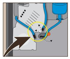
4 Remove the delivery tube on the left and the coffee tube directly next to it, and allow them to hang down loosely. Turn the product delivery bracket to the right and lock it in place.
