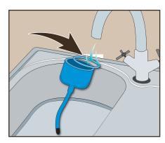
Use a cleaning brush to clean the light blue mixer and use a narrow brush to clean the delivery hoses. Thoroughly dry the mixer. Reassemble the parts in reverse order.
