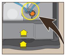
8 Reinstall the drip pan and coffee grounds container. Screw in the orange screw cap, turn the product delivery bracket to the left and insert the delivery tubes.
