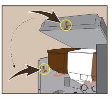
Remove the service key and close the machine again.
