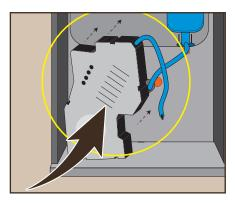
7 Clean the internal coffee strainers under running water and then reinstall the brewer in reverse order between the red retaining clips.
