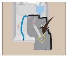
6 Push the bolt for the crank drive on the back of the brewer clockwise downwards.
