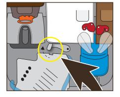
Push the brewer's retaining brackets upwards.
