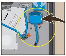
Fully release the light blue hose at the delivery outlet. Remove the complete mixer and tube forwards.
