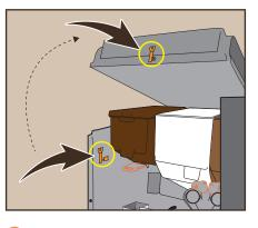
Remove the service key from its holder on the left wall of the housing and start up the machine.
