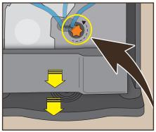
2 Remove the coffee grounds container and drip pan, and unscrew the orange screw cap.
